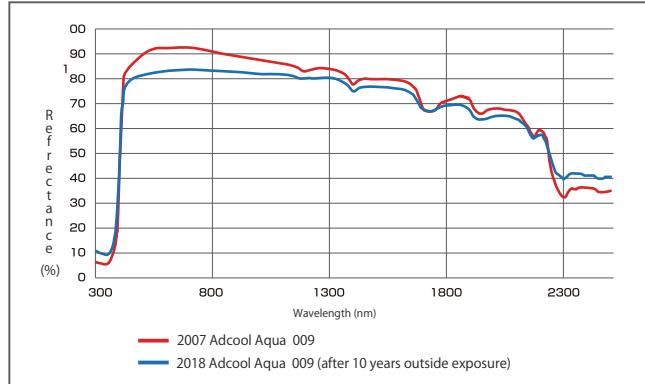
Even after the 10 years, Adcool Aqua keeps approximately 90 % of the reflectance tremendously.
